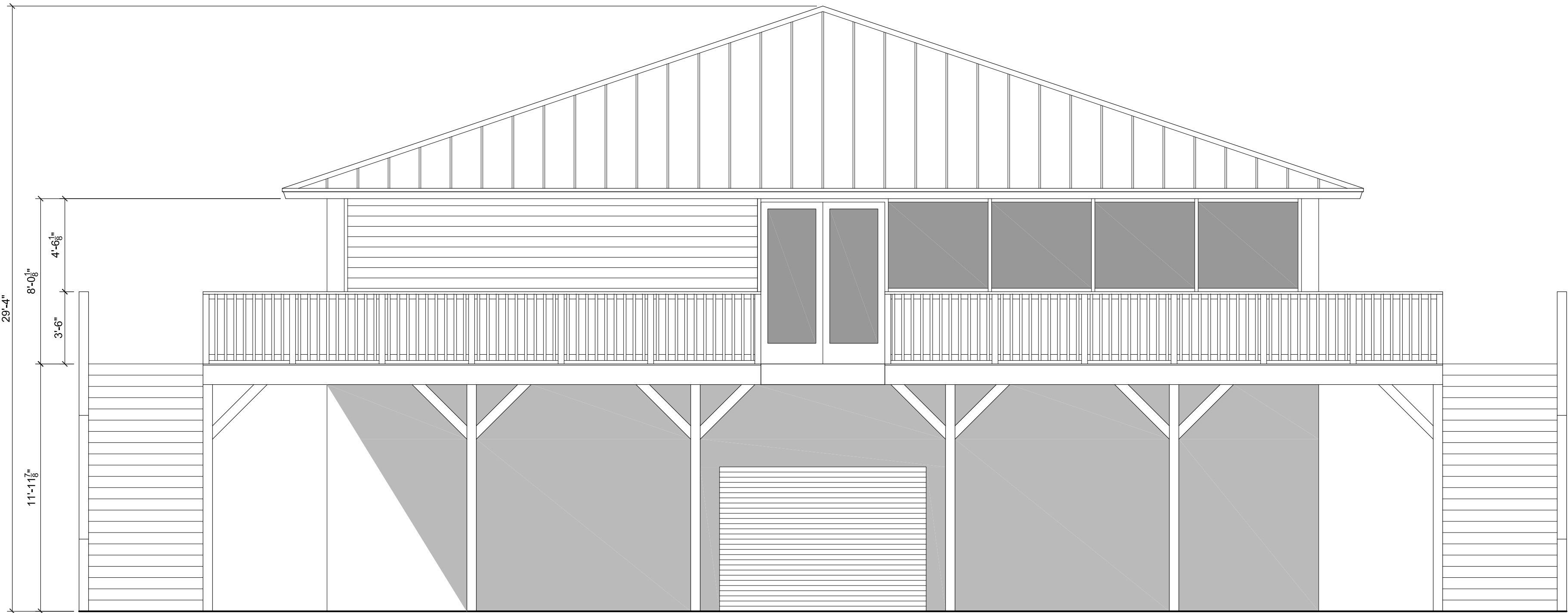
1 PROPOSED NORTH ELEVATION SCALE: 1/4" = 1'-0"
